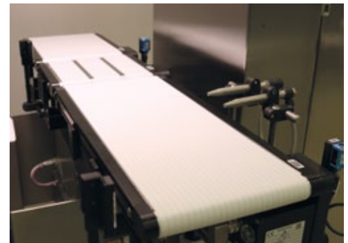
Air blast nozzle (on the right) for secure ejection of under or overweight products
