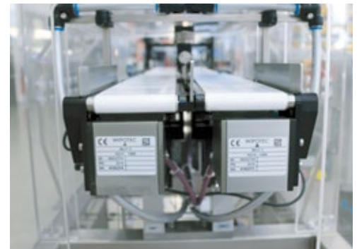
State-of-the-art HC-A weighing technology as multi-track option
