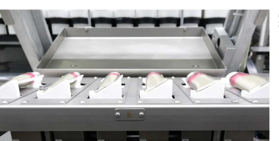
Pick & Place inline weighing as a cost-effective alternative to belt scales
