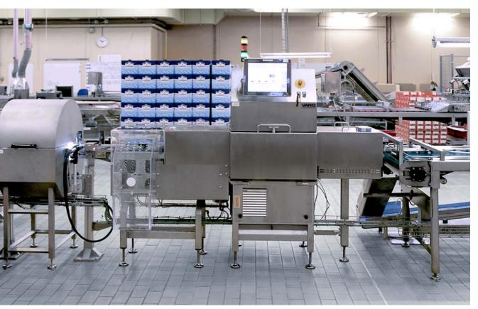
Canned mackerel: production line with integrated X-ray inspection system
