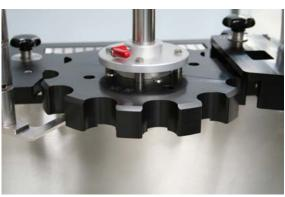
A star wheel with format-specific pockets, picks up the products as they arrive on the conveyor belt and rotates the product over the Weigh Cell.
