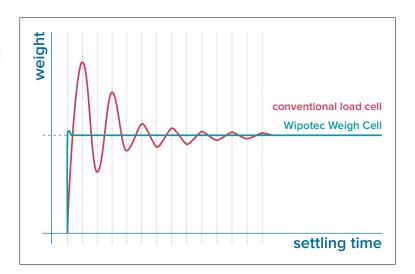
caused by drive units of machines or due to imbalance forces, making them potentially useful for all manufacturers. It shows that Weigh Cells with AVC sensors can be used cross-sectorally to measure product weights accurately. The patented AVC technology is a black box. The precise mechanical design and the algorithms working in the background are proprietary WIPOTEC company technologies.
