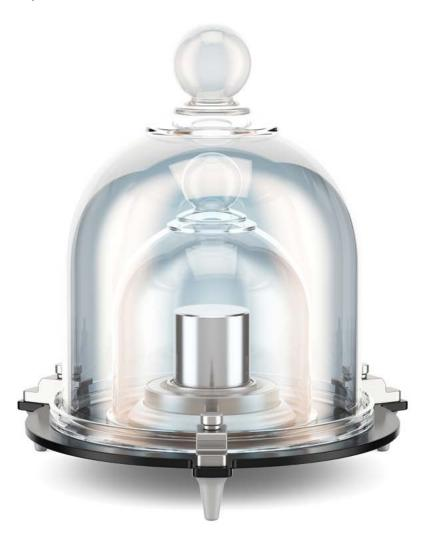
ntil recently, all goods weighed – from tablet blister packs to bulk goods – brought an additional 50  $\mu$ g per kilo more to the scales than the scales showed on the display. The reason for this discrepancy, which in practice is hardly dramatic, was that the International Prototype of the Kilogram (IPK) has lost weight over the past 100 years. So, if the scales showed one kilo, in fact the object weighed slightly more because the IPK always weighs exactly one kilo. This does not mean that the
