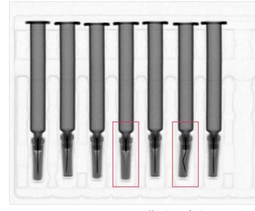
X-ray image of syringes, left: missing needle, right: bent needle
