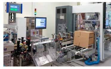
TQS-HC-A with an integrated checkweigher for fully automated serialisation and completeness check on the smallest footprint
