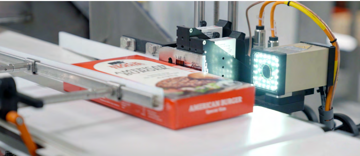
The printer and camera work together.
