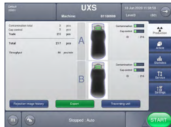
X-ray image of a bottle from two different sides
