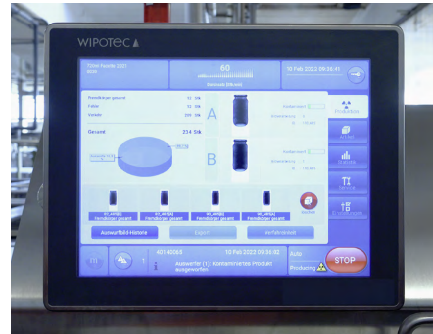
The 15" HMI shows the X-ray images of the beet jars
