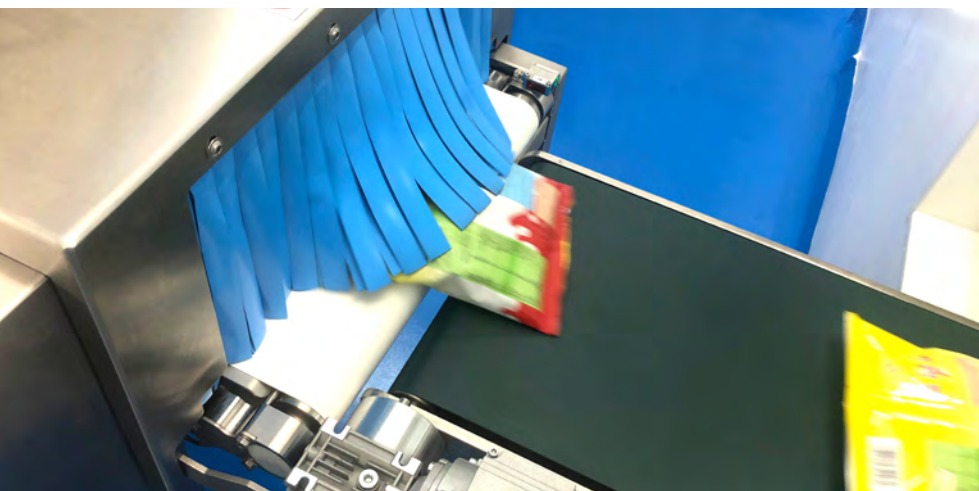
Radiation protection is vital: "Rino" milk powder at the discharge spout of the SC-E 4000
