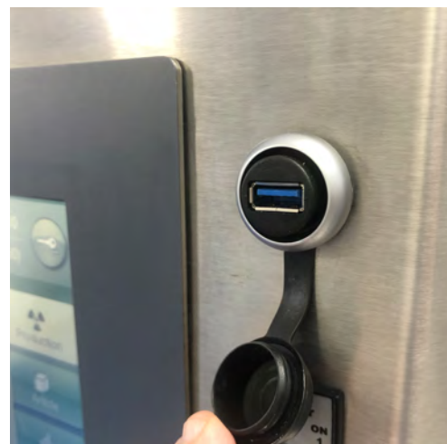
USB interface on the X-ray scanner: for backups, statistics and many other applications
