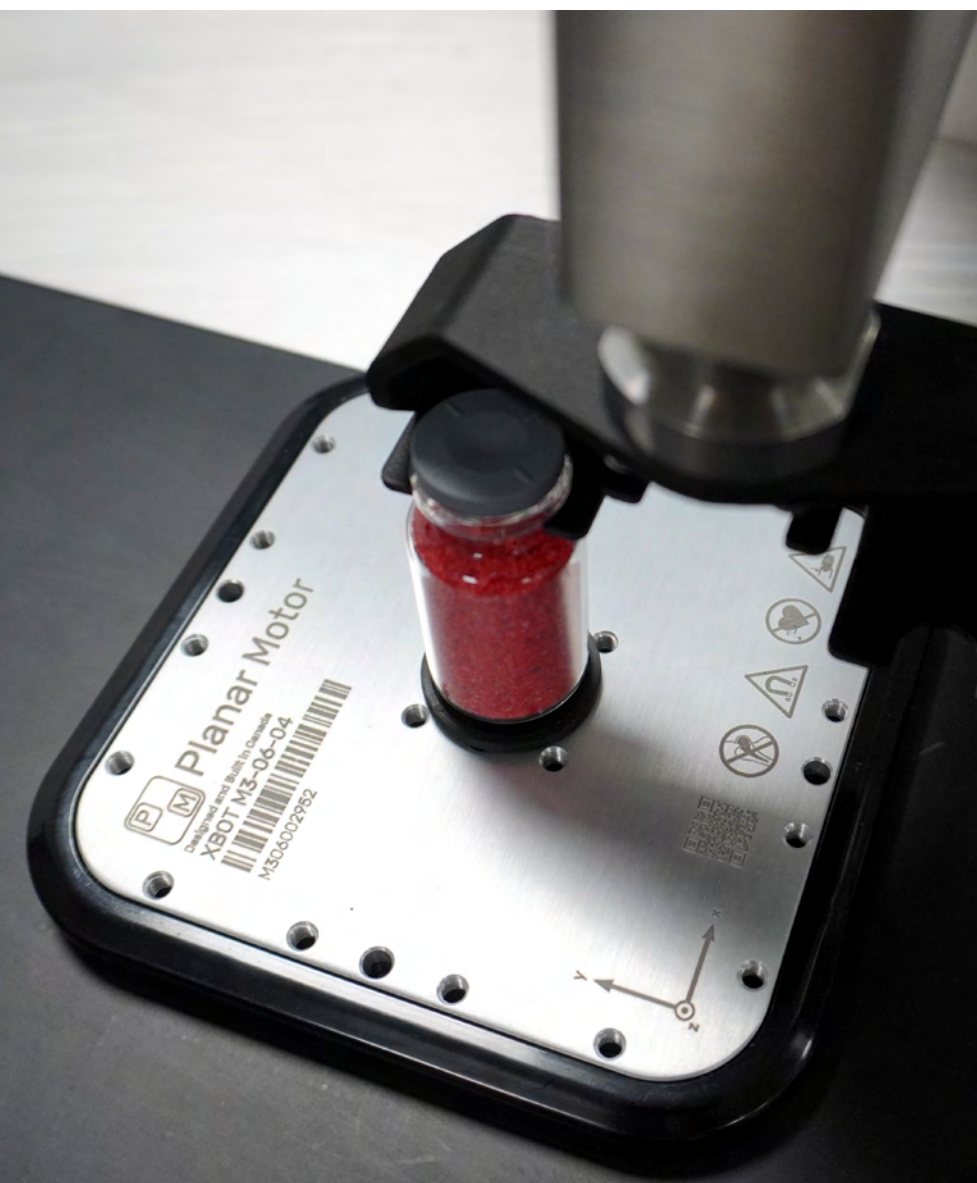
Positioning of the product on the weigh cell
